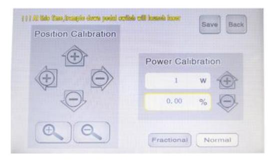
Power Calibration: Checked , select the power value to be calibrated, and then select , adjust the value and use the laser power meter to measure the actual power of the laser at this time, so that "display value of power to be calibrated" = "maximum power of laser" × "percentage of actual power to be calibrated", please save it before exiting.
