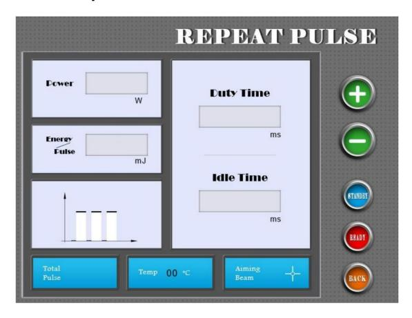
Use the parameter button to adjust, control the laser output power to be 0-30W
