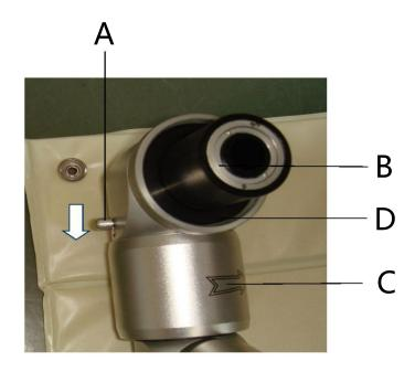
Rotate end B toward the direction indicated by end C in the picture by 180 degrees, and the circlip of end A in the picture will automatically lock in the direction indicated by the picture (if it returns to the original position, turn the circlip of end A to the direction indicated in the picture) , and then insert the B end into the main body base. Finally, lock the lock nut D of the light guide arm.
